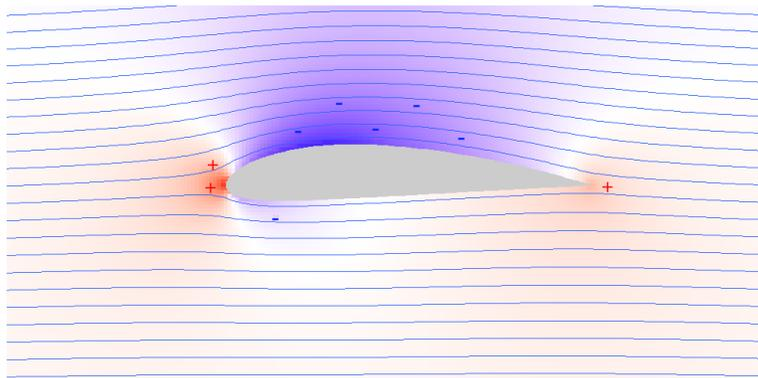
The geometry of the airfoil is such that the bottom is almost flat, while the top is more curved than the corresponding symmetric airfoil. Consequently, the streamlines (even at zero angle of attack) exhibit more curvature at the top than at the bottom, compared to the symmetric airfoil at zero angle of attack. As illustrated in the figure, the pressure is consequently lower at the top than at the bottom, and net lift is generated.
