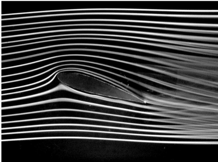
We notice that the streamlines from top and bottom of the airfoil join smoothly at the trailing edge, and leave it in a direction tangent to the chord of the airfoil, thus inclined downwards. The corresponding simulated flow, including the pressure differences from ambient, is as follows (two streamlines close to the surface of the airfoil are highlighted for emphasis).
