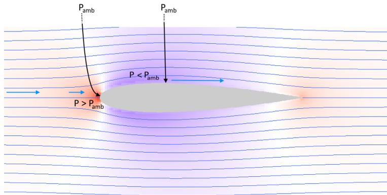
(The blue arrows represent air velocity—by Bernoulli's law, the velocity will be lower in the region of relatively high pressure around the leading edge, and higher in the region of relatively low pressure on top of the airfoil).
