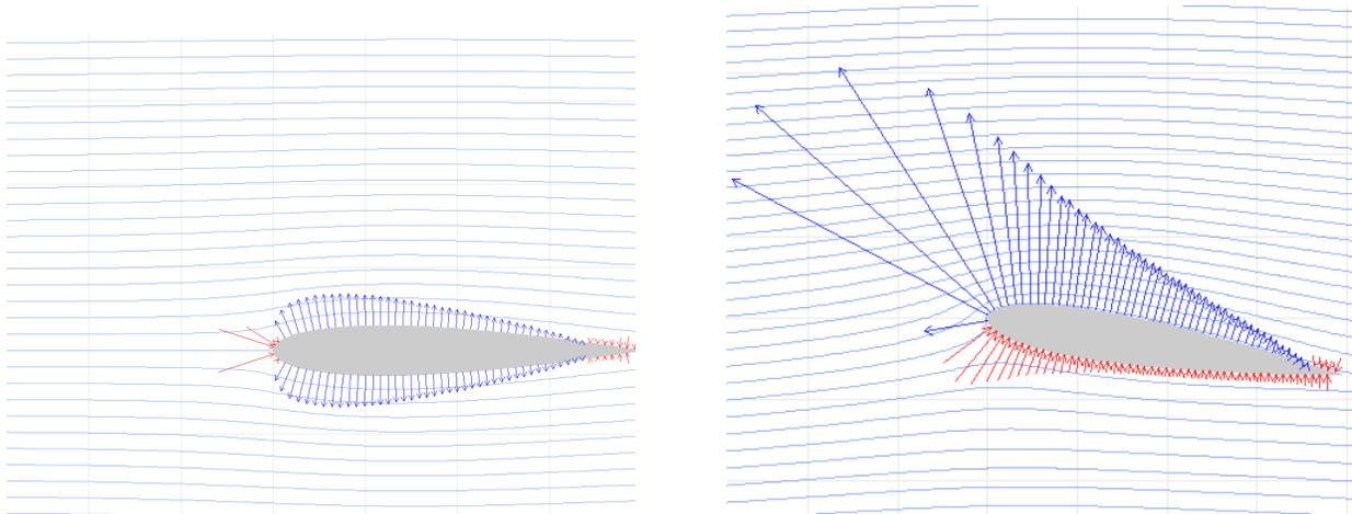
What about a non-symmetrical airfoil? Let's have a look at a cambered airfoil more typical of a general aviation aircraft, placed at zero angle of attack..
