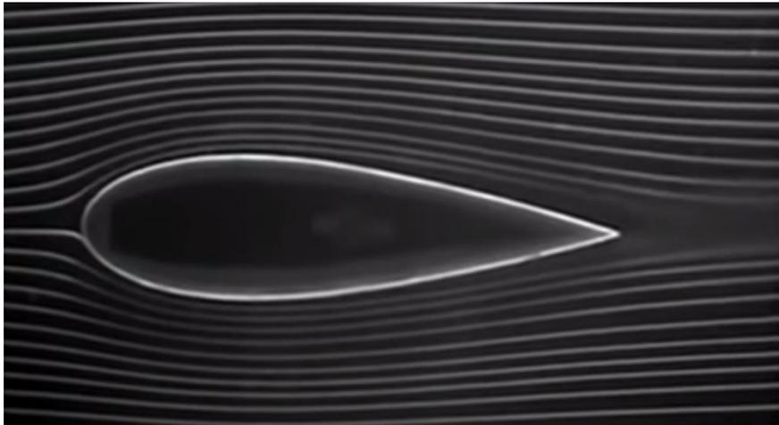
In the absence of any obstacle, the streamlines would be equidistant horizontal lines. The presence of the airfoil forces the streamlines to part away shortly upstream of it, and they rejoin downstream. Far from the airfoil, the streamlines are mostly undisturbed from uniform flow, but close to it, they curve to follow the contour.
